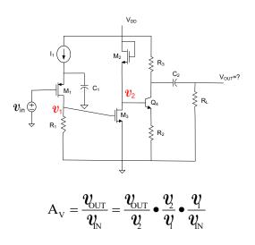
The last state is a CE with RE stage. The middle stage is a CS stage and the first stage is a CS stage. Thus from the last state
